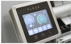
Automatic vertical alignment control panel
